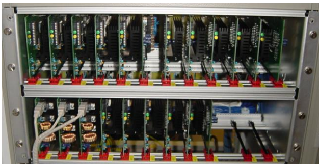
Example: 3 Stations of 5 axes each controlled via 3 independent USB channels.
